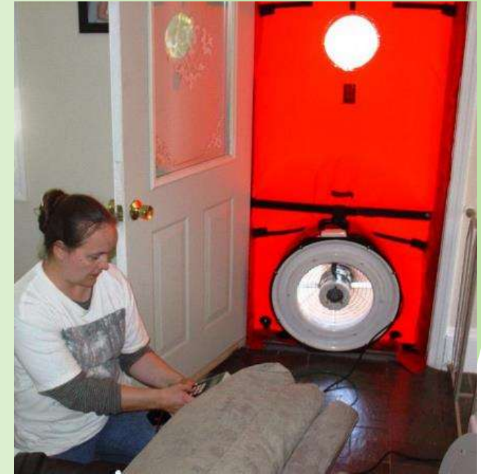
Blower door tests now Energy Code-required
